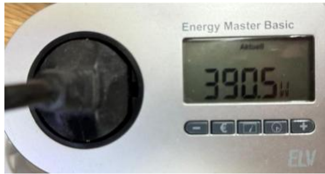
Figure 3: Power Meter (ELV Energy Master): Measured Minimum Load: 390.5 W
