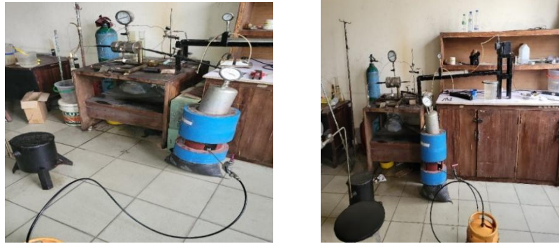
Figure 1,2: Core Flood set – up (Chemical (Left) ; Steam (Right))
