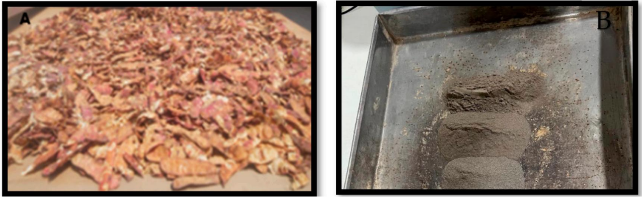
Figure 1: (A) Dried tara husk collected and selected as the base material for ash production. (B) Sample of tara ash obtained after calcination, ready to be sieved and used as an additive in the concrete mix design.
